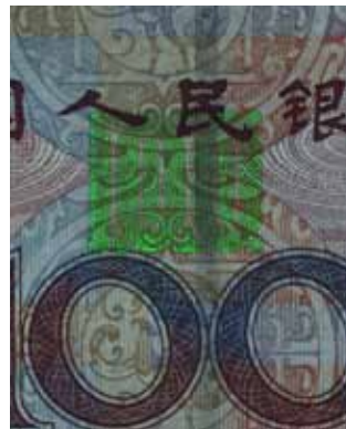
Wide-band visualization of «anti-Stokes inks»
