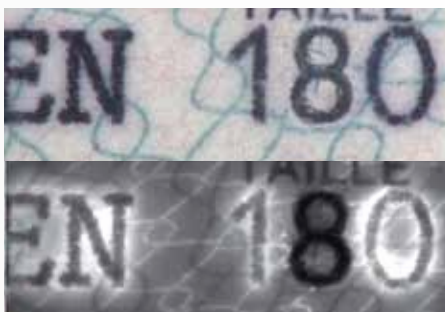
IR luminescence investigation to differentiate printing inks
