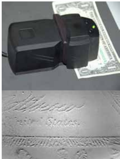
Magnetic Ink Detector: Detector to visualize magnetic ink in documents
