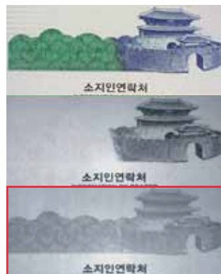
Comparative illustration with IR absorption; above: original in visual light, middle: IR 850 nm absorption, below: forgery
