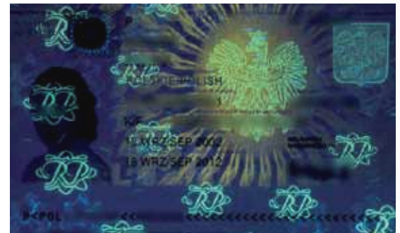
Security features in UV 365 nm
